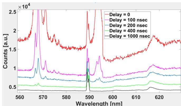
Figure 3: LIBS measurements on a running water jet
