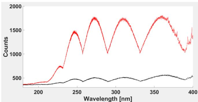
Figure 5: CMOS response with UV coating (red) and without coating (black)
