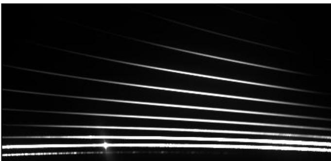
Figure 1: Typical echelle image of the IRIS spectrometer
