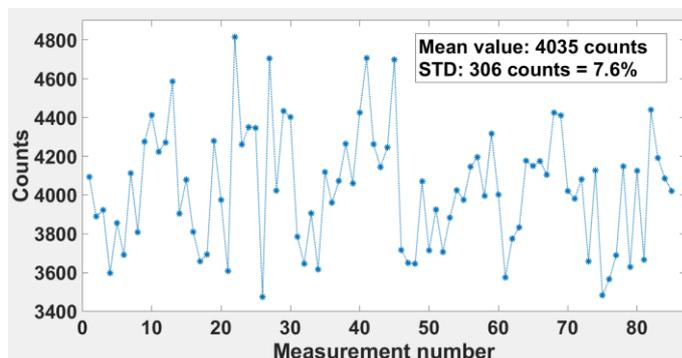
Figure 4: Sequence of 85 single shot LIBS measurements. Counts are the peak height of an iron peak measured on a flat steel sample.
